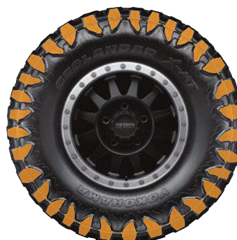
Wide Lug Groove satisfies with Off-road Traction.
